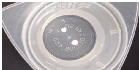
Figure 4 - An intact, stable emulsion on the water's surface
